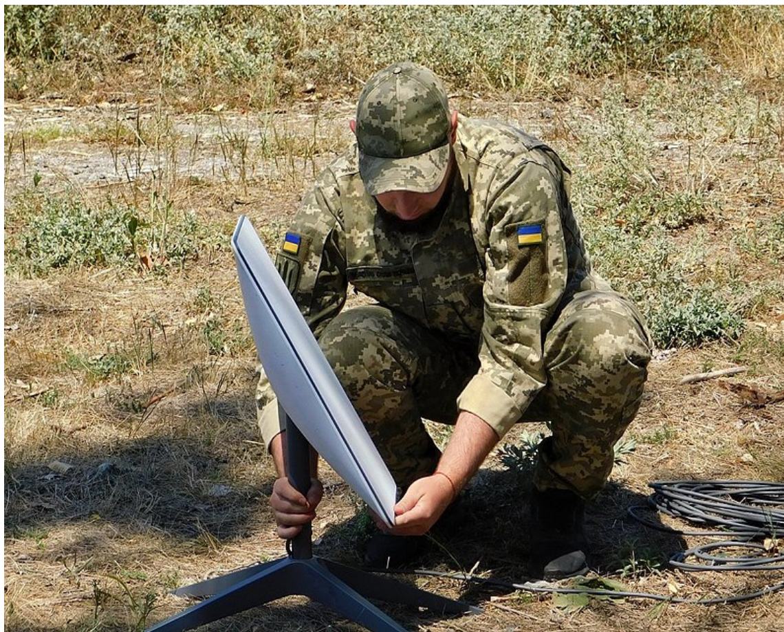
Figure 1: A Ukrainian soldier installing a Starlink user terminal 7
