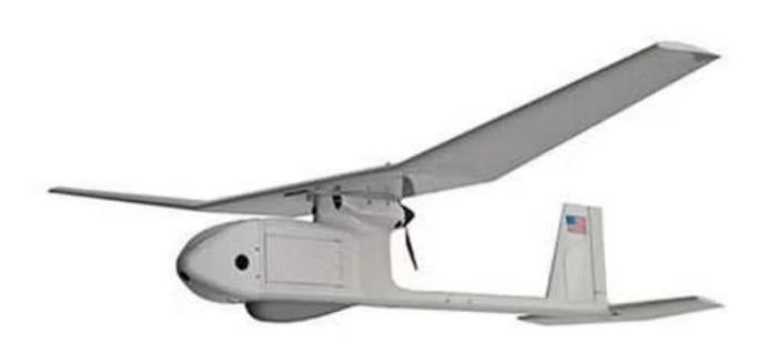
Fixed-wing UAVs are like airplanes, using wings and forward motion for efficient, long-distance flight. However they cannot hover and often need a runway or launcher. Some noteable examples include the Chinese Wing Loong II, Turkish Bayraktar TB-2, and the indigenous GIDS Shahpar.<sup>5</sup>
