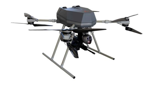
Rotary-wing UAVs use spinning blades for vertical takeoff, hovering, and agile maneuvering in any direction. They are ideal for close-proximity tasks but usually with shorter flight times. Pakistan's rotary-wing UAVs include the Asisgard Songar and the domestically produced GIDS Ranger. <sup>4</sup>
