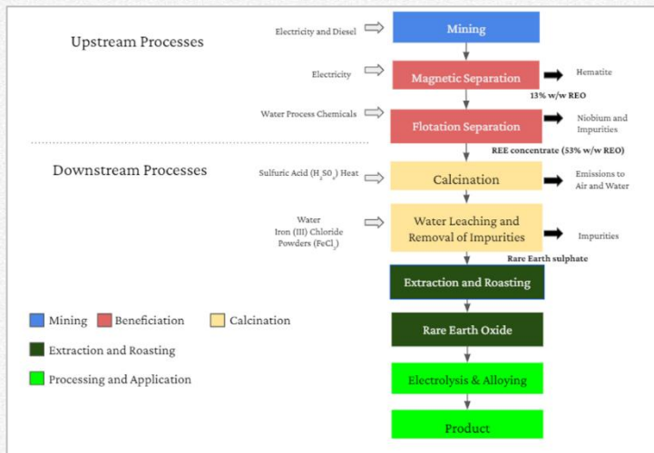
Process diagram for the extraction of REEs.
